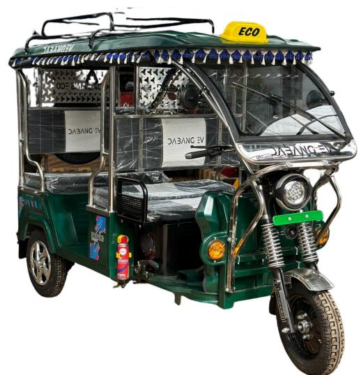
DABANG ECO SS COMES WITH A DURABLE STEEL BODY, POWERFUL 1200W MOTOR, 140AH BATTERY, AND A RANGE OF 110+ KM BUILT TOUGH FOR HEAVY-DUTY ELECTRIC MOBILITY.
